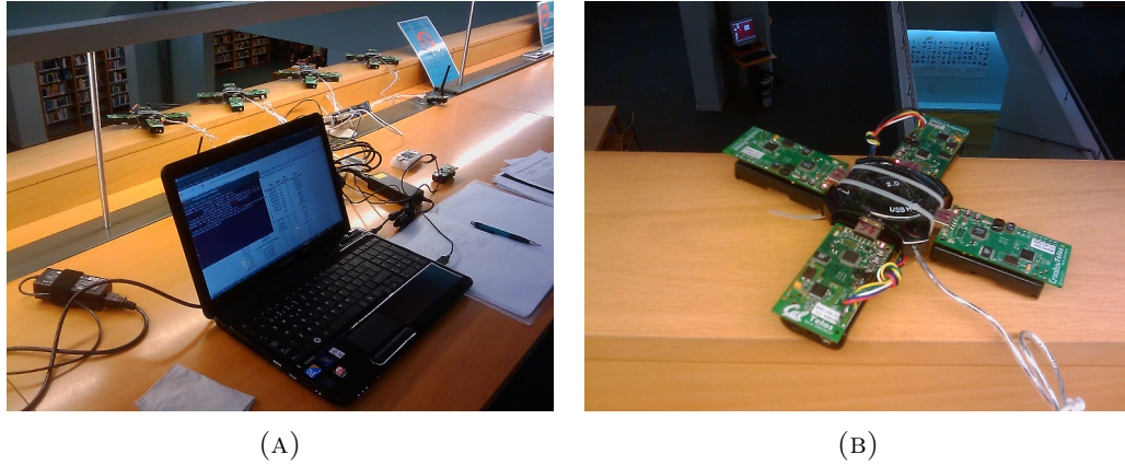
FIGURE 3.2: The experimental setup used to collect energy level traces on IEEE-802.15.4 channels deployed at the Library of the Faculty of Engineering at the University of Porto (a) and detail of TelosB motes arranged in a USB hub (b)
