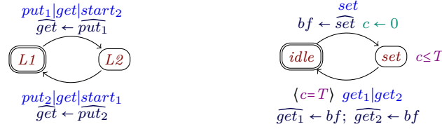
Figure 3: The composed THA for the running example in Fig. 2 (left), and the composed Timer and Duplicator example from section Section 2.3 (right).
