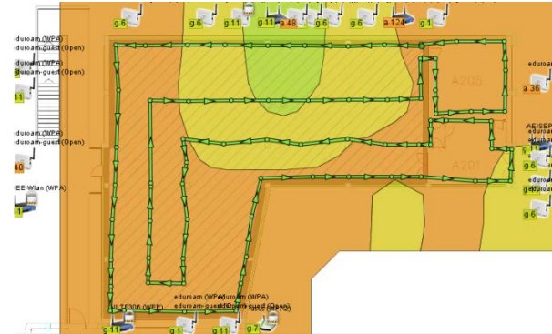
Figure 11 - DEMMON1 Deployment – ISM spectrum (namely, WLAN) interference study in the site's area
