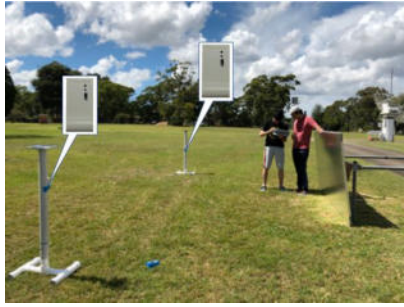
(a-1) CIR measurements at the outdoor open field.
