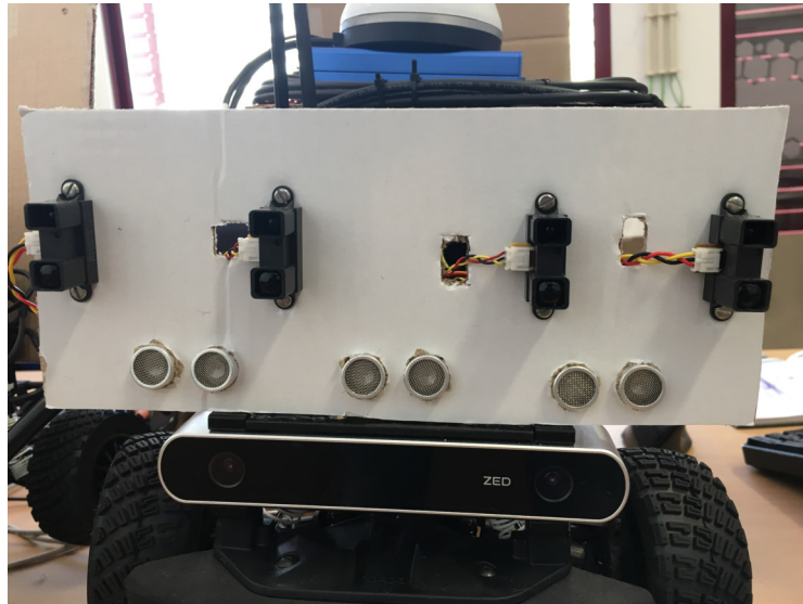
Figure 5.8: Sensor Control Board
